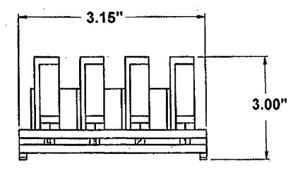
Coil leads are the "bussed common" type which means that one side of each coil is connected to a common bus on the module. In this configuration a single wire back to common is all that is requited for all four relays on a given module. This saves time and simplifies wiring.
