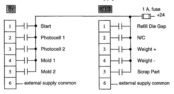
Note the installation of the fuse to protect the external power supply in the event of a short circuit in the wiring or a malfunction in the programmer. Note too that the fuse rating has been increased to a 1 amp fast blow fuse because it is now supplying all 10 inputs.
