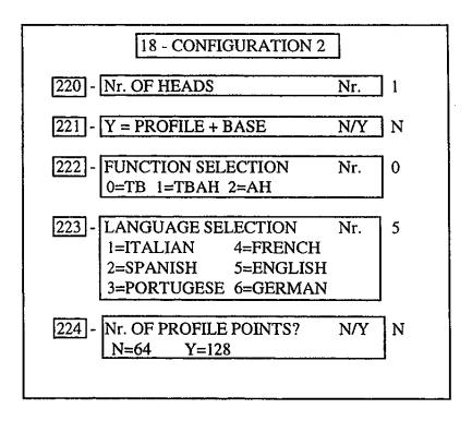
220 - Nr. OF HEADS Using the numerical keypad, select the number of active parison heads from 1 to 4. Owing to the limited capabilities of heads 2, 3, and 4 this version programmer is mostly used on single head machines and so will usually be set to "1".
