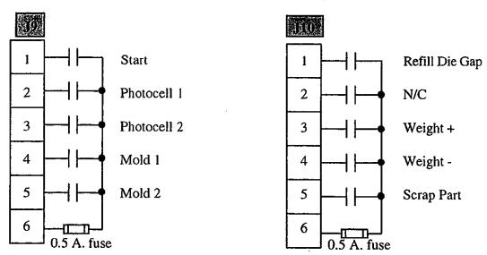
Power for each of the terminal blocks is available at terminal #6. If more than two or three inputs in total are used, it is recommended splitting the source between the two terminal blocks to provide more even loading of the power supply.
