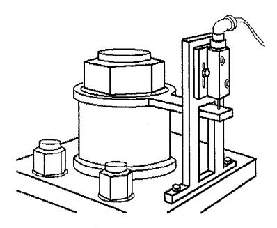
Note the provisions made for vertical adjustment of the DCDT body and the antirotational arrangement incorporated to keep the core and body aligned.
