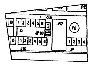
If an external 24 volt source for power to the inputs is used, the **JP 10** jumper should be positioned VERTICALLY (90 degrees to that shown in the drawing).
