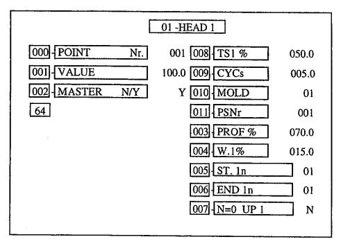
Each data field is preceded by a three digit reference number to help in identifying a specific field and function.
